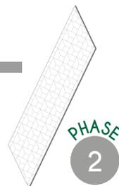
Membrane composed of 2 layers of polypropylene woven and interposed a fiber-glass mesh. It distributes evenly the tensions deriving from the foundation and allows the absorption of dimensional variations between backsurface and tile. TEXTILE is applied on the whole surface between the first and the second layer of GENIUX glue.
